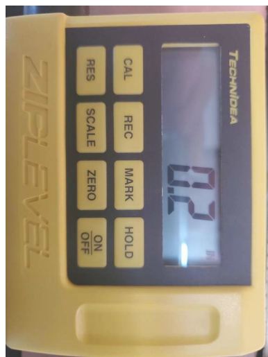
.2" of slope from left to right across entire foundation.
